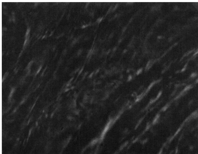
Fig. 2. Photograph of polarized light transmitted from a thin layer of a 12% solution poly( p -phenyleneterephthalamide) in 100% H 2 SO 4 ; 23°C. 185×.
